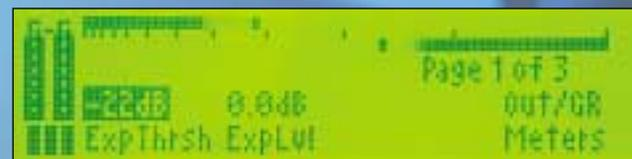
Dynamics level meters show I/O levels, gain reduction, peak expansion.
